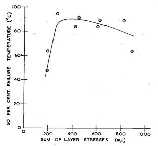
Fig. 10. Effect of layer stress on thermal endurance of miniature valves
