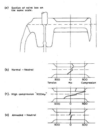
Fig. 7. Retardation gradients resulting from various strain-setting arrangements
