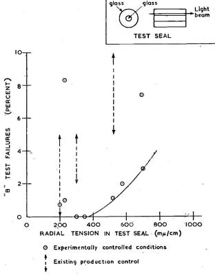
Fig. 3. Dependence of minimum failures 'B' test on degrees of mismatch
